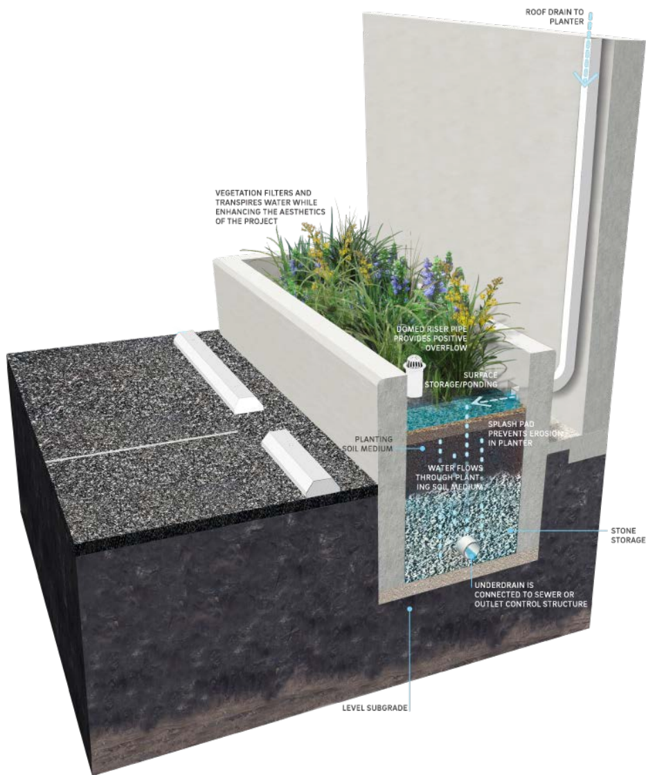
Figure 48. Construction of a bioretention planter ( https://www.pwdplanreview.org/manual/chapter-4/4.1-bioinfiltration-bioretention )
