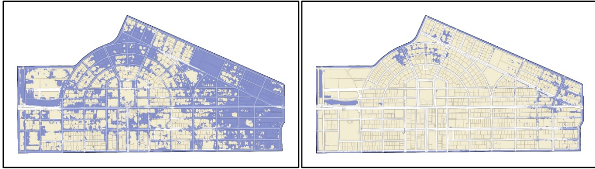
Figure 108. Results of screening tool flood modeling before (left) and after (right) simulating installation of the pumping station (areas shaded in blue correspond to those properties that are flooded during the 3-day, 25-year storm event)
