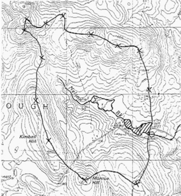
Figure 3. An example of a USGS topographic map used to define a watershed. ( https://www.nrcs.usda.gov/Internet/FSE_MEDIA/nrcs144p2_014463.jpg )
